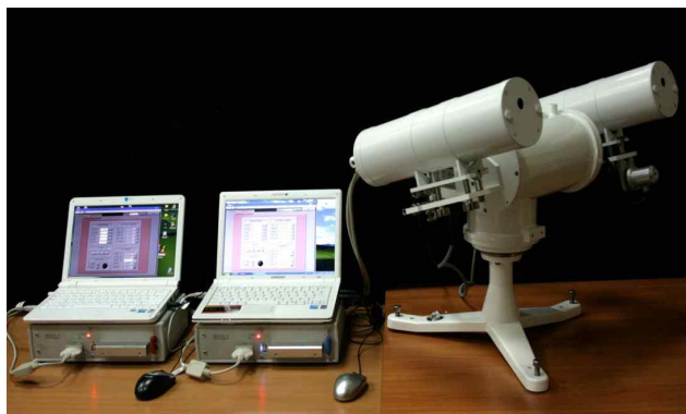
Figure 17. Appearance of two modified radiometers MAR-1 installed on the Sun tracker STR 22.
