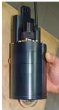
Figure 1. Overall external view of the miniaturized multi-spectral “CE-600” underwater fish-eye radiance camera (joint development by LOV and CIMEL Electronique).
