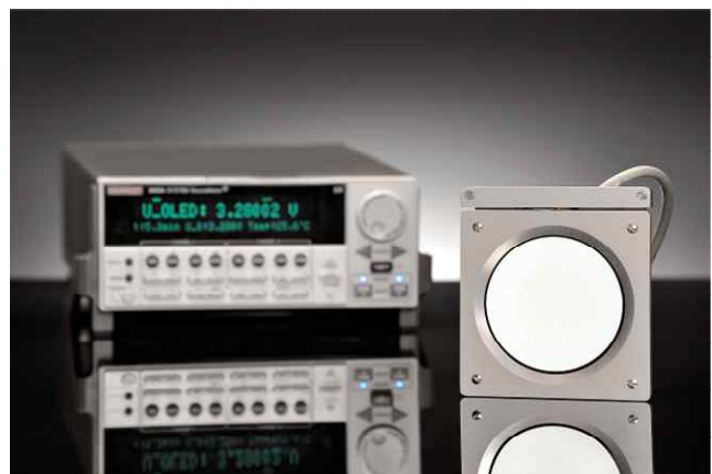
Figure 25. Temperature stabilised OLED transfer standard and power source.
