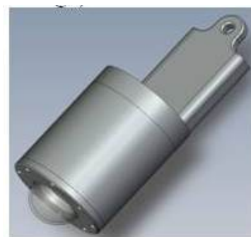
Figure 1. Overall external view of the miniaturized multi-spectral “CE-600” underwater fish-eye radiance camera (joint development by LOV and CIMEL Electronique).
