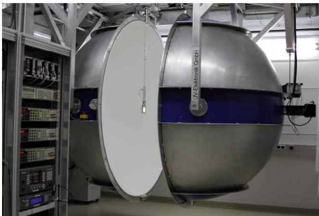
Figure 26. OLED transfer standard mounted in a temperature stabilised 2.5 m diameter integrating sphere.
