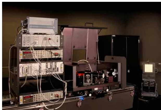
Figure 21. PTB bench carriage with several optical and electrical measurement devices and a large area OLED mounted on a turning device.
