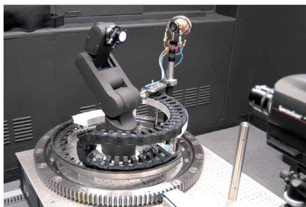
Figure 2. Photo of the setup of the robot-based gonireflectometer at NRC.
