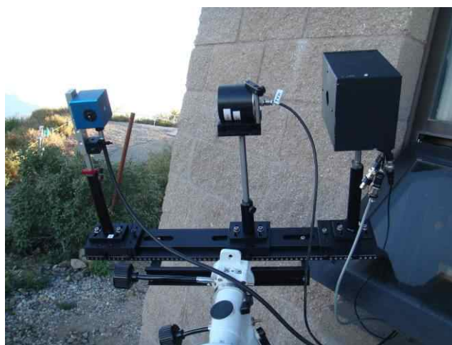
Figure 1. Prototype of the calibration source mounted on a rail and tripod on Mt. Hopkins summit. The black box on right contains a 2 inch integrating sphere, shutter, and light source. The blue cube at left is the irradiance calibration head. A removable LED for initial alignment with the telescope is in between. The spectrometer and electronics are inside the window at right.
