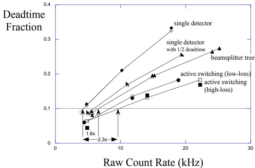
Fig. 6. Measured (solid points) and calculated (open points connected by lines to guide the eye) DTF versus the overall count rate on InGaAs for different detection arrangements.
