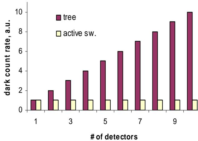
Fig. 3. Dark count rates for  $N$  detector arrangements in units of a single conventional detector.
