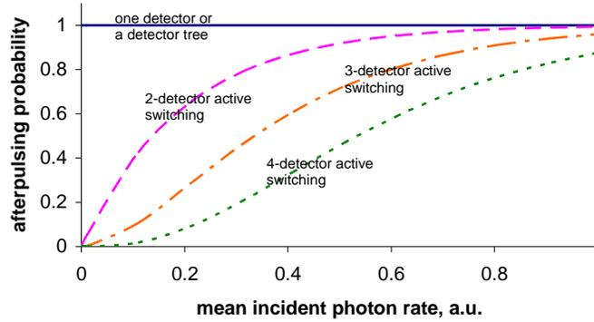
Fig. 4. Afterpulsing probability rate for an active switching multidetector arrangement with two (dashed line), three (dotted-dashed) and four detectors (dotted) and for a single detector or a tree arrangement (solid).
