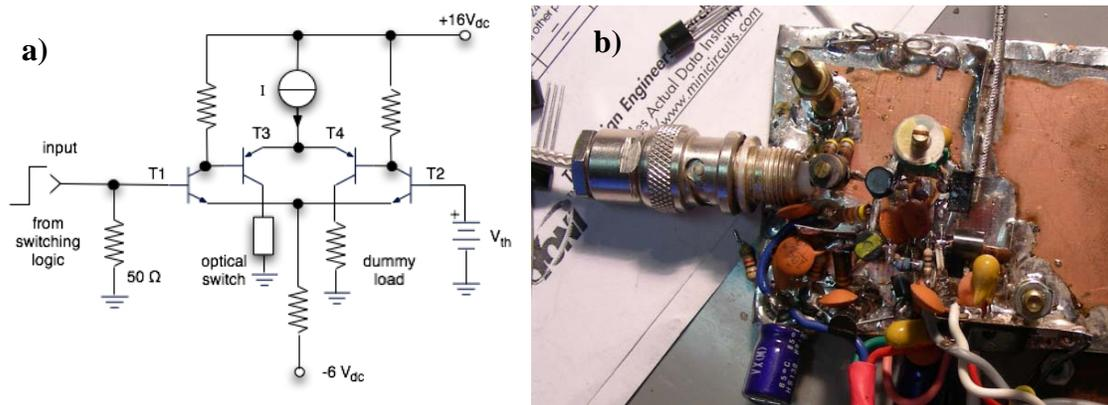
Fig. 7. Optical switch electrical driver a) schematic and b) prototype.
