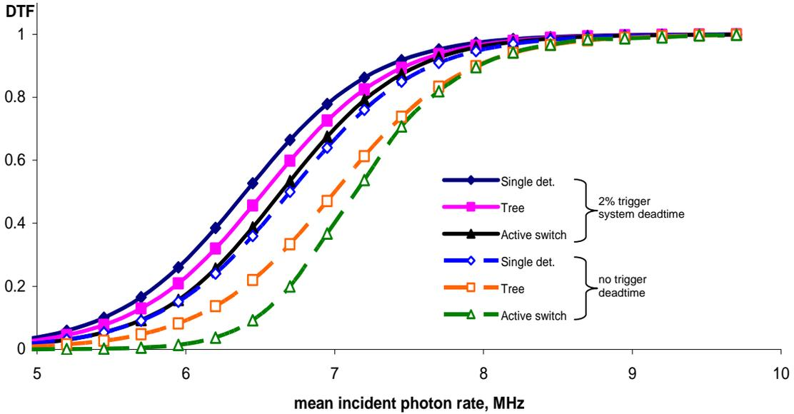
Fig. 2. Effect of nonzero trigger system deadtime on DTF for various detector arrangements of 1 and 2 detectors. Diamonds: single detector; squares: tree arrangement; triangles: actively switched arrangement; open markers: no trigger system deadtime; filled markers: trigger system deadtime  $T_t = 0.02 T_d$ .
