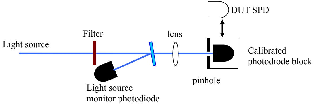
Fig. 2. Calibration setup.
