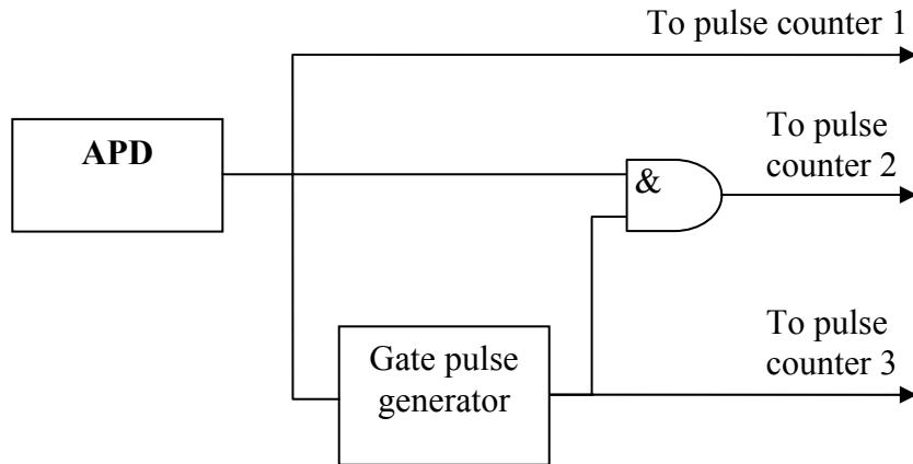
Fig. 4. Schematics of a setup to measure an electronic afterpulsing fraction and an effective twilight time.
