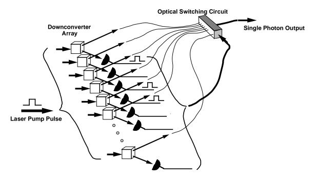
**Figure 1.** General schematic for single photon source showing array of crystal downconverters each with the potential of producing a pair or pairs of photons. The each downconverter is shown with its own trigger detector. The information about which trigger detectors have fired is sent to the optical switching circuit to control which incoming lines are directed to the output line. Input line delays to allow the trigger information to arrive before the incoming photons are not shown.
