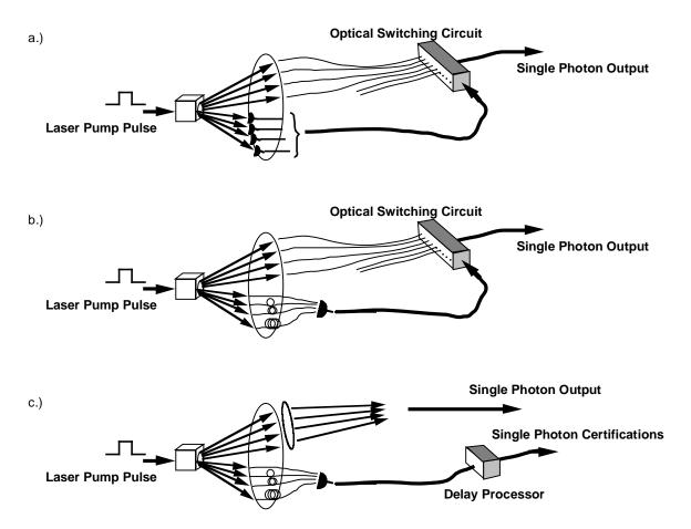
**Figure 2.** a.) Single crystal implementation of scheme. b.) Single detector implementation of scheme. Sequential series of delay lines is seen leading to the trigger detector. c.) Implementation without the optical switching circuit. A lens is used to collect all the modes correlated to those seen by the trigger.
