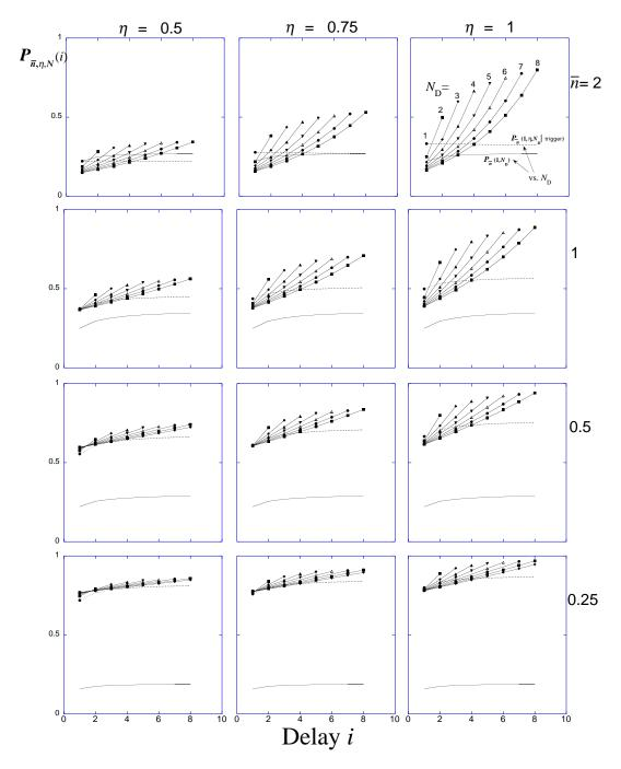
**Figure 4.** Matrix of graphs single photon probabilities similar to fig 3a for a range of values of  $\overline{n}$  and  $\eta$ . The columns correspond to  $\eta$ 's of 0.5, 0.75, and 1 from left to right, while the rows correspond to  $\overline{n}$ 's of 2, 1, 0.5, 0.25 from top to bottom.
