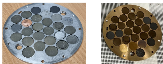
(a) Holder pre-irradiation (b) Holder post-irradiation Fig. 1: Photo of the ACT holder pre- and post-irradiation
