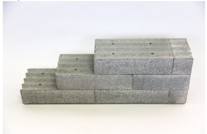
Fig. 1: Low-activity concrete bricks developed for shielding. Typical activities are ^{226}\text{Ra} \approx 0.6 \text{ Bq/kg} , ^{228}\text{Th} \approx 0.3 \text{ Bq/kg} and ^{40}\text{K} \approx 6 \text{ Bq/kg} .
