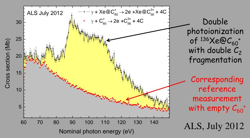
Optimization of the operating parameters and use of isotopically enriched  $^{136}$ Xe in the synthesis increased the Xe@ $C_{60}^+$  ion beam current by more than an order of magnitude!
