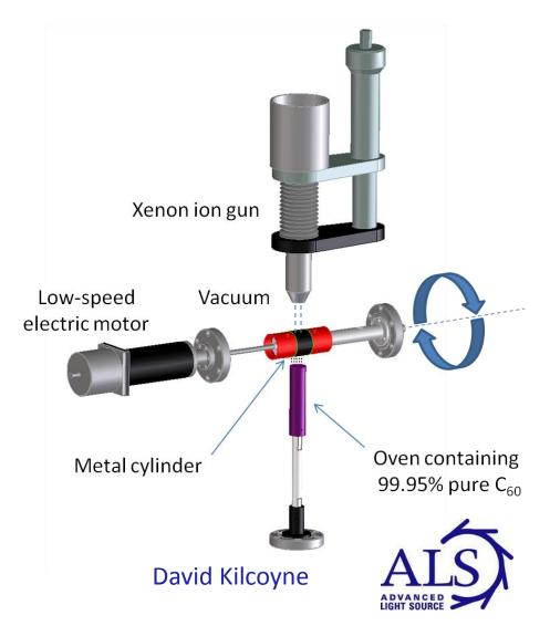
Ultra-high-purity commercial  $C_{60}$  powder was continuously evaporated and deposited onto a rotating metal cylinder while it was being simultaneously bombarded by 160 eV Xe<sup>+</sup> ions.
