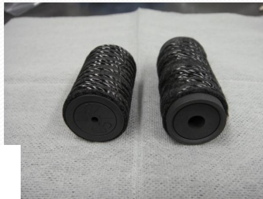
High-Temperature Fixed Point (HTFP) cavities Courtesy Y. Yamada
