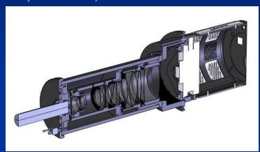
Resonon Volume Phase Holographic (VPH) in line spectrograph
