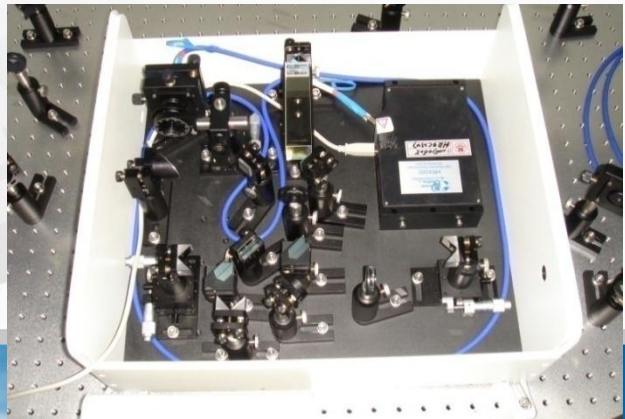
Experimental setup of SPIDER
