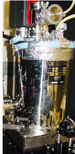
Laser Optimized Cryogenic Radiometer (LOCR) 1990s
